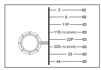
Figure 5. Stator Assembly Leads
